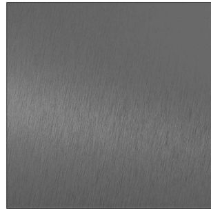
5. ALUMINIUM POWDER COAT WINDOWS SATIN CHARCOAL GREY 25 MICRONS
